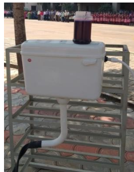
Mechanical Cylinder and Piston based Toilet Liquid Sanitizer Dispenser (February 2021)
